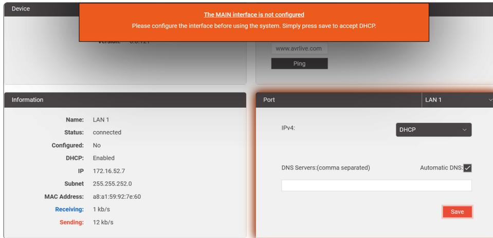
3. If connected to a DHCP enabled network click save in the "Port" window. Refer to "[Port Configuration](#)" on page 9 for configuration of static IP settings.
